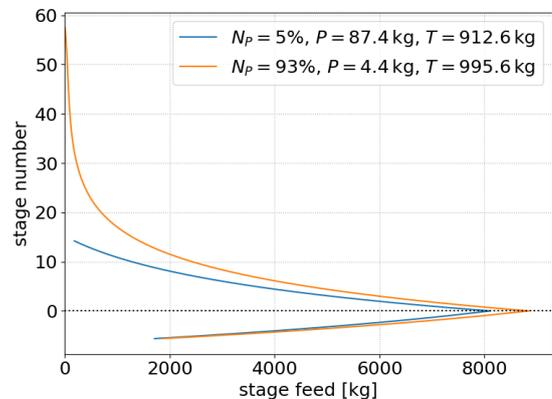
Figure 1: Material flow per stage in an ideal enrichment process
