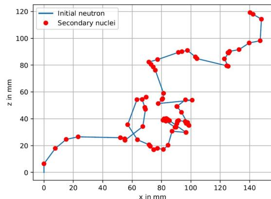
Figure 2: A trajectory of a neutron in the Time Projection Chamber, which was produced by an antineutrino interaction.
