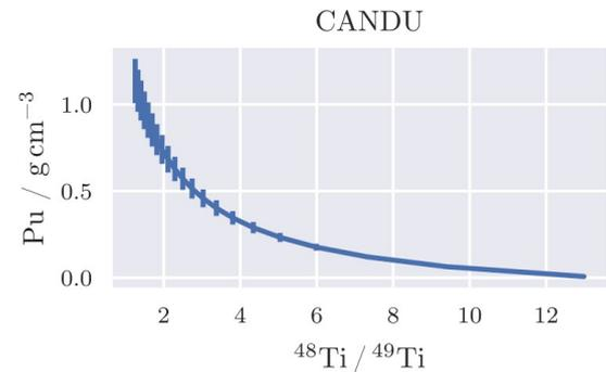
Figure 3: Determining the plutonium production using the isotopic ratio of Ti-48 and Ti-49 in a CANDU nuclear reactor
